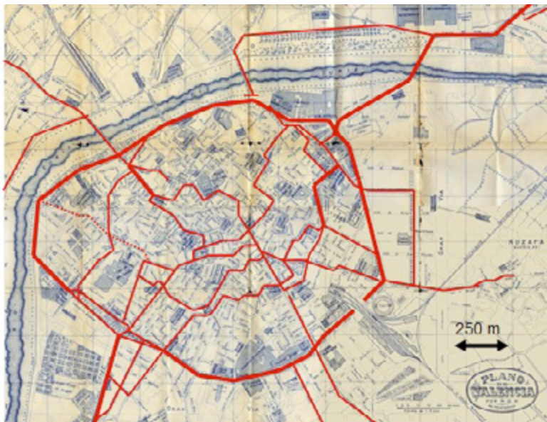
Figure 2.4. Map of the city of Valencia. Tram lines in 1898 underlined in red. Gross lines denote double track and narrow lines single track. Dotted line corresponds to a link open to public service later. Imprenta Ortega's map from Collection Huguet.
